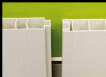
▲ Easy fit tongue and groove join for fast installation and demounting. Pre-finished 300mm wide x 30mm thick pvc panels. (stocked lengths in selected increments from 2.4m to 6m.)
